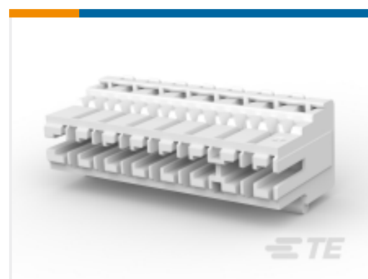
TE Part # 1703128-1 8POS MT - EDGE HOUSING
